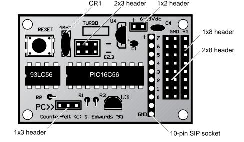
U1—93LC56 serial EEPROM (may substitute 93LC66) in 8-pin DIP socket
